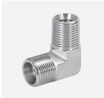
P/N:1CN9 90°NPT male /metric male 24°cone l.t
