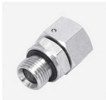
P/N:2BC-WD BSP thread with captive seal/metric female 24° cone o-ring sealing
