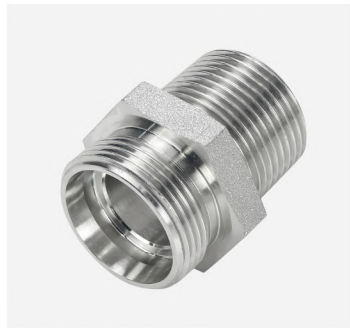
P/N:1CT BSPT male /metric male 24° cone l.t
