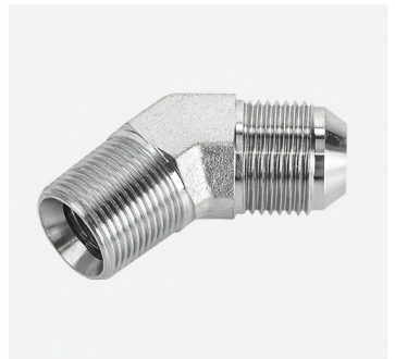
P/N:1JT4 45°elbow JIC male 74° cone/BSPT male
