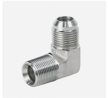
P/N:1JT9 90°elbow JIC male 74° cone/BSPT male
