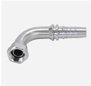
P/N:22693 90° bsp female 60° cone interlock fitting
