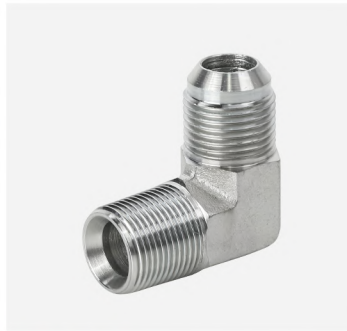
P/N:1JN9 90°elbow JIC male 74° cone/NPT male
