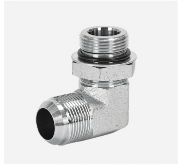
P/N:1JO9 90°elbow JIC male 74°cone /sae o-ring
